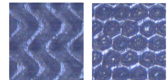
Figure 4. Surface structure for UniCorr and b) anilox roll 355 l/cm at 100 times magnification
