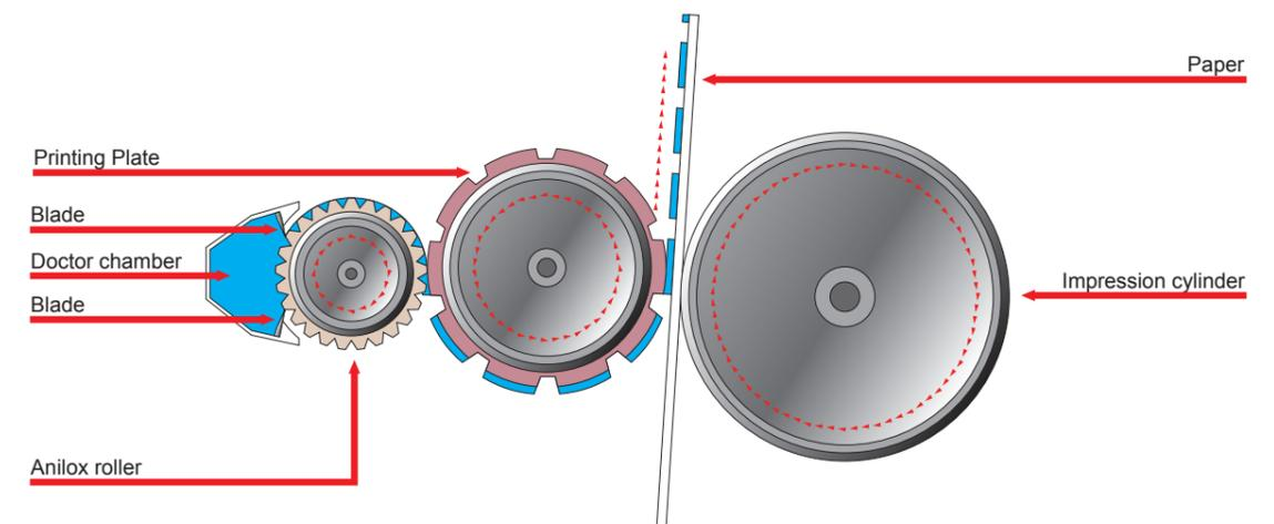
Figure 3. The major components in ink transfer using the flexographic central impression cylinder printing.
